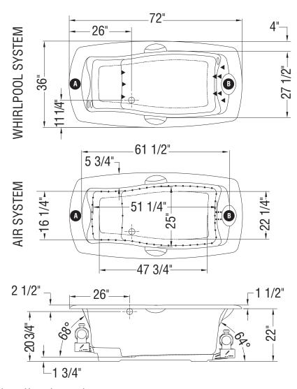
Note: A or B pump location could exceed by one in. on combo.
