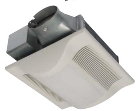
WhisperValue-Lite ENERGY STAR rated performance-valued exhaust fans with light fixtures feature totally enclosed AC condenser motors for long-life and energy efficiency. These low file models have a 3 3/4" height, operates with 4" round compatible oval duct, and comply with green building IAQ standards. Two 18-Watt compact fluorescent lamps and one 4-Watt night-lamp are included with an ENERGY STAR light fixture.
