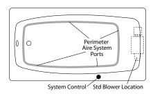
Sump Dimen: 48" long x 23-1/2" wide x 17-1/2" deep Sump Capacity: 52 gal. (unoccupied - to overflow)
