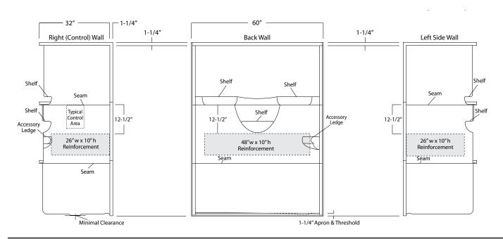
Package Order No.: TLRF-LS (RH drain-LH seat reinforcement)
