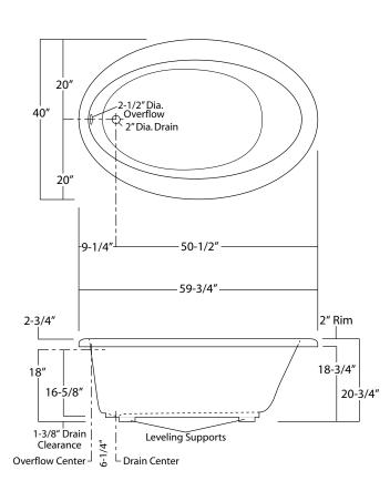
Sump Dimen:47" long x 27" wide x 18-1/2" deepSump Capacity:62 gal. (unoccupied - to overflow)Whirlpool Operating:40 gal.
