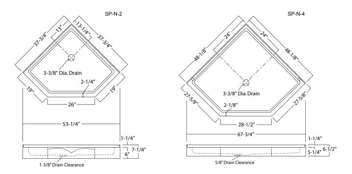
**NOTE**: Critical enclosure dimensions should be taken directly from the installed shower base with finished wall surround. Dimensions shown above for dam are <u>NOT</u> centerline door dimensions
