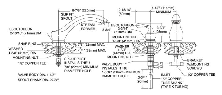
NOTE: THE INSTALLATION SHOWN IS FOR TILE DECKS, THIS VALVE WILL ALSO FIT STEEL, CAST IRON OR PLASTIC DECKS
