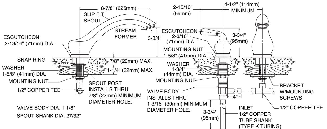
**NOTE:** THE INSTALLATION SHOWN IS FOR TILE DECKS, THIS VALVE WILL ALSO FIT STEEL, CAST IRON OR PLASTIC DECKS
