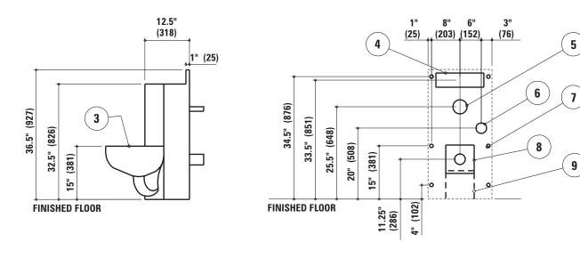
Right hand fixture is shown. Left hand fixture is reversed.
