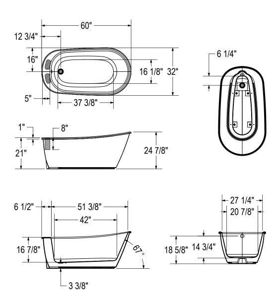
(:)): Recommended faucet area 2 sections of 7" (L) x 3" (W). Depth recommended for straight pipes 8".
