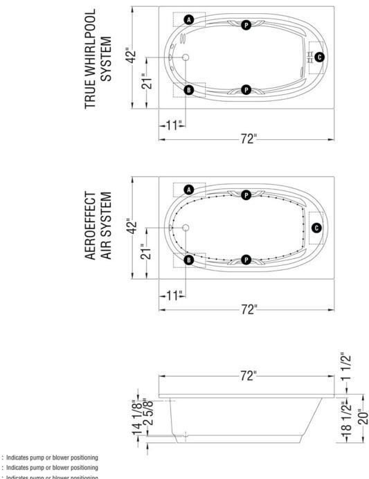
0 0 : Indicates pump or blower positioning G : Indicates pump or blower positioning 0 : Indicates optional grab bars positioning
