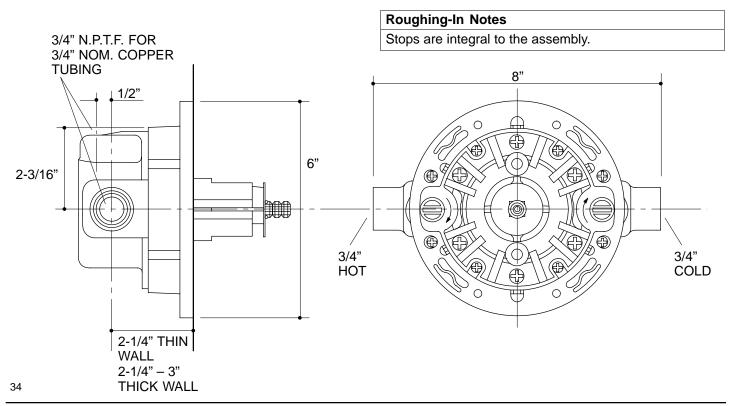
**K-306-KS** HiFlow Rite-Temp™ Pressure-Balancing Valve 117229-1-**CC**
