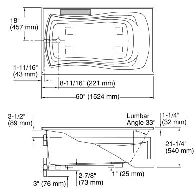
No changes in measurements if connected with drain illustrated. (K-7161-AF)
