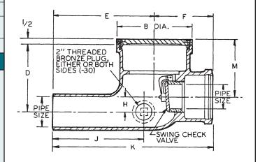
**NOTE:** SWING-CHECK VALVE NORMALLY HANGS IN CLOSED POSITION, BUT CAN BE SET TO HANG OPEN.
