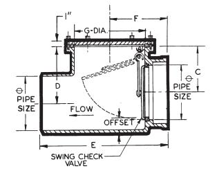
**NOTE:** SWING-CHECK VALVE NORMALLY HANGS IN CLOSED POSITION, BUT CAN BE SET TO HANG OPEN.
