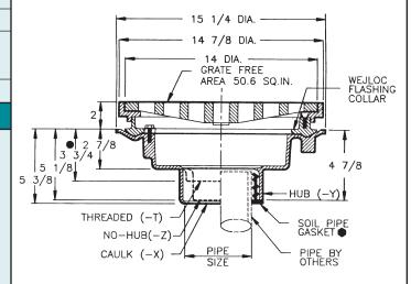
CONFORMS WITH ASTM-C564.THIS DIM. IS 5-3/4" FOR 34718-T.
