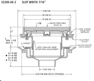
CONFORMS WITH ASTM-C564.
