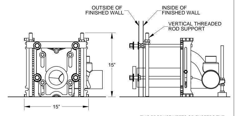
RECOMMEND CONCRETE ANCHORS WITH 750 LBS. PULL-OUT FORCE EACH.
