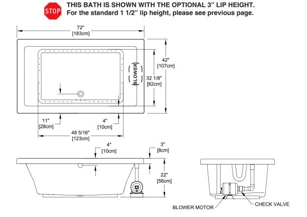
NOTE: To accomodate customer preferences, the control keypads are not factory installed on the bath deck. A six (6) foot cable with installation instructions for connecting the control keypad to the control box are provided with all baths. Patents recieved or pending. Note: Dimensional Tolerances: +1/4"
