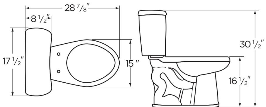
THIS FIXTURE QUALIFIES ACCORDING TO ASME TEST PROCEDURES AS A LOW CONSUMPTION WATER CLOSET WITH AN AVERAGE CONSUMPTION OF 1.6 gpf (6 Lpf) OR LESS.
