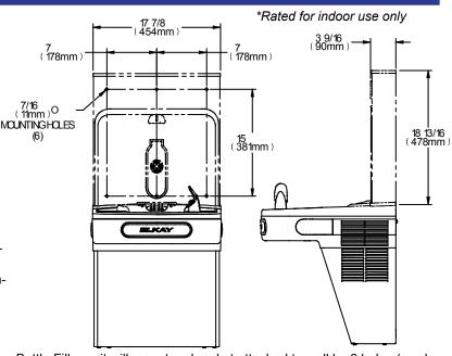
Bottle Filler unit will mount on bracket attached to wall by 6 holes (as shown). Water and electrical will connect through pre-punched hole in basin.
