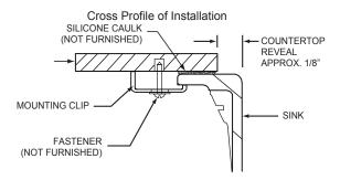
Cross Profile of Installation For Sinks Purchased Prior To Apr. 1, 2013 Template 74180592
