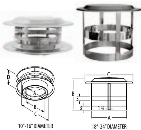
Required where pipe terminates above the roof line. Removable screws allow for cleaning of the chimney and spark arrestor screen. Made of stainless steel.
