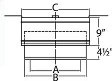
Supports chimney pipe and provides a positive connection between support box and chimney with a built-in twist-lock. Supports up to 40' of DuraTech Chimney. Trim collars are sold separately. (For 10" use DuraBlack Slip Connector to attach DuraBlack to the support box. See DVL/DuraBlack section).
