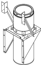
Use as wall support for chimney system. Use of straps is optional. Supports up to 50' of DuraTech Chimney without straps, and 70' of DuraTech Chimney with straps. Attaches to chimney pipe. Can be installed above or below the Tee. If installed below the Tee, a short section of pipe is required. Adjustable base provides 2" to 6" clearance to wall.
