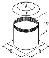
Use in installations that pass through an attic to prevent insulation and debris from accumulating near the chimney, unless chimney is enclosed through attic. Fits over Firestop Radiation Shield or a support box. Consists of two parts – a collar and a base. Mesh sleeve around top.
