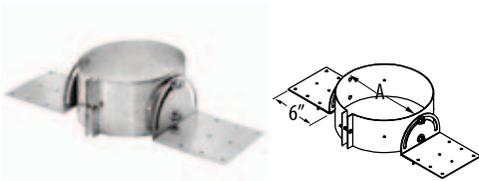
Designed to support the DuraTech Chimney and allows the chimney to pass through the roof and extend down from the ceiling. Ideal for cathedral ceilings and free-standing fireplace installations. Supports up to a maximum total chimney length of 45' above and 20' chimney below Roof Support. Adjustable to different roof pitches. Use Finishing Collar and adapter to attach DVL or DuraBlack to the DuraTech chimney. Trim Collar not included.
