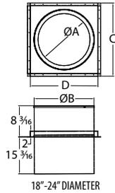
Use in ceiling/floor penetrations other than those that include the ceiling support. Fits on underside of ceiling and adjusts to cover framing.
