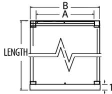
**10" - 24" Diameters** - Designed for appliances that are tested and listed for use with a 1700° F rated chimney system, such as zero-clearance or masonry fireplaces, furnaces, boilers, water heaters, ranges, or other appliances fueled by oil, coal, gas, or wood. Tested to UL 103 and listed under MH 7399. Available in galvalume (GA) and stainless steel (SS) outer wall and stainless steel inner wall. Requires fastening with screws.
