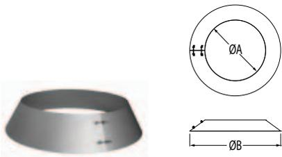
Required with DuraTech flashing to create a weather-proof penetration through the roof deck. Seal inner edge of the collar to the chimney pipe with non-hardening 500° F high-temperature sealant.
