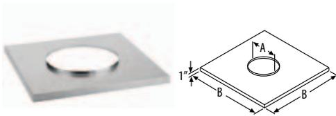
Encloses the top of a chase while providing a ventilation air passage from the chase. UL Listed. Includes spacer clips. Storm collar not included. Made of galvalume.
