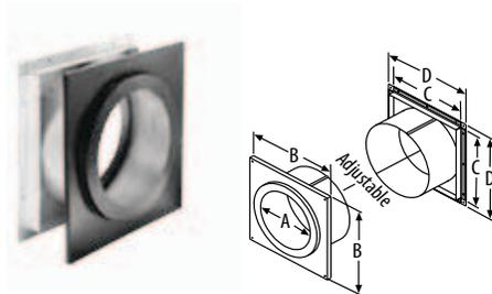
Adjusts from a minimum of 4" to a maximum of 10" wall thickness, and fits between standard wall studs. To accommodate thicker walls, the telescoping pieces can be extended up to 16" with a field-fabricated extension installed. Interior trim ring painted black. Must be installed with DuraTech chimney pipe horizontally through the wall and extend 6" into the room beyond the interior wall. (Black painted DuraTech is available). 6" and 8" stainless steel exterior trim available.
