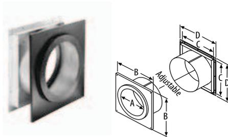
Use to provide clearance to combustibles. Adjusts from a minimum of 4" to a maximum of 10" wall thickness, and fits between standard wall studs. To accommodate thicker walls, the telescoping pieces can be extended up to 16" with a field-fabricated extension installed. Interior trim ring painted black. Must be installed with DuraTech chimney pipe horizontally through the wall and extend 6" into the room beyond the interior wall.
