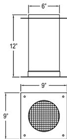
Allows required ventilation air into chase. Screen keeps rodents out.
