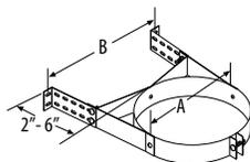
Use in interior or exterior installations to add lateral support to the chimney. Assures a 2" to 6" clearance to combustible walls. Required every 8'.
