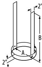
Use to prevent excessive weight on the elbows by supporting the weight of the chimney. Required to be installed between two elbows in offset installations. Multiple elbow straps may be required for offset installations. Refer to installation instructions.
