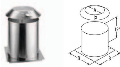
Required for installations that pass through an attic to prevent insulation and debris from accumulating near the chimney. Fits over Firestop Radiation Shield or a support box. Consists of two parts – a collar and a base.
