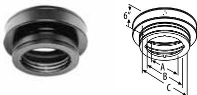
Supports chimney pipe and provides a positive connection between support box and chimney with a built-in twist-lock. Supports up to 60' of DuraTech Chimney. Use adapter to attach DVL or DuraBlack to the support box. Painted black. Trim collars are sold separately. (For adapters see DVL/DuraBlack section.)
