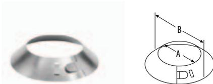
Required with DuraTech flashing to create a weather-proof penetration through the roof deck. Seal inner edge of the collar to the chimney pipe with non-hardening 500° F high-temperature sealant. Made of aluminum.
