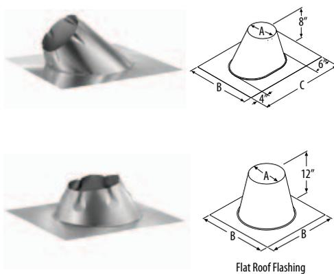
Use to weather proof the penetration of chimney pipe through the roof. Storm Collar required. Select roof flashing based on pitch of roof. For example, a 6/12 pitch has a vertical rise of 6" over a horizontal distance of 12". Made of galvalume.
