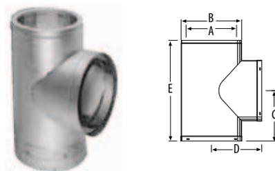
Use for through-the-wall installations. Includes removable Tee Cap for easy chimney cleaning or inspection. Wall Straps, a Wall Thimble, and an Adjustable Tee Support Bracket must be installed with the Tee as directed. Available in stainless steel or with a galvalume outer wall and stainless steel inner wall. See installation instructions for proper location and installation of Tee.
