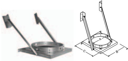
Use as wall support for chimney system. Supports up to 30' of DuraTech Chimney. Attaches to chimney pipe. Can be installed above or below the Tee. If installed below the Tee, a short section of pipe is required.
