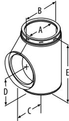
Use for through-the-wall installations. Includes removable tee cap for easy chimney cleaning or inspection. Wall Straps, a Wall Thimble, and an Adjustable Tee Support Bracket must be installed with the Tee as directed. Available in stainless steel or with a galvalume outer wall and stainless steel inner wall. See installation instructions for proper location and installation of Tee.
