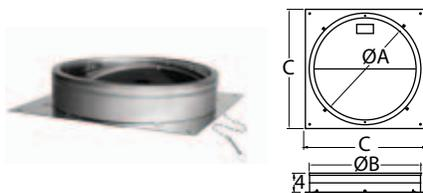
Use as a starter section for DuraTech. Bolts directly to fireplace outlet. Damper section allows chimney to be closed when fireplace is not in use. Includes chain and lintel hook.
