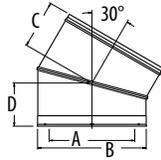
Use for offsets around obstructions such as rafters, ridgepoles, or joists. May have one pair of elbows if needed. Offsets greater than 30° are not permitted in accordance to UL 103 standards. Large diameters are restricted to one pair of elbows.
