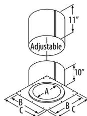
Use in ceiling/floor penetrations when a ceiling support is not used. Not required when passing through the roof. Fits on underside of ceiling and adjusts to cover framing.
