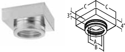
Supports chimney pipe and provides a positive connection between support box and chimney with a built-in twist-lock. Designed for installation in flat ceilings only. Supports up to 60' of DuraTech Chimney. Use adapter to attach DVL or DuraBlack to the support box. A 2" wide trim collar is included. Not painted, but can be painted with high temperature paint. (For adapters see DVL/DuraBlack section).
