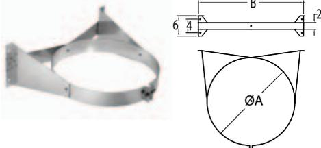
Use in interior or exterior installations to add lateral support to the chimney. Assures a 2" clearance to combustible walls. Required every 4'.
