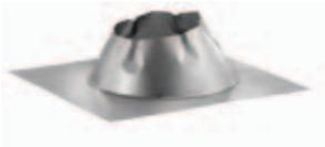
Use with metal or tile roofs. Available in sizes 6" and 8" in large base 0/12-6/12 (shown) and 7/12-12/12 styles. Made of dead soft aluminum. Refer to Roof Flashing table for dimensions.
