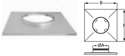
Encloses the top of a chase while providing a ventilation air passage from the chase. UL Listed. Includes spacer clips. Storm collar not included. Made of galvalume.
