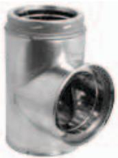
Use for through-the-wall installations. Includes removable tee cap for easy chimney cleaning or inspection. Wall Straps, a Wall Thimble, and an Adjustable Tee Support Bracket must be installed with the Tee as directed. Available in stainless steel or with a galvalume outer wall and stainless steel inner wall. See installation instructions for proper location and installation of Tee.
