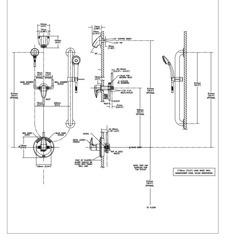
Delta reserves the right (1) to make changes to specifications and materials, and (2) to change or discontinue models, both without notice or obligation. Dimensions are for reference. Measurement may vary plus or minus 6mm(0.25"). Mounting locations are suggested only. Check with local codes for requirements in your area. This spec was produced August 16, 2012.
