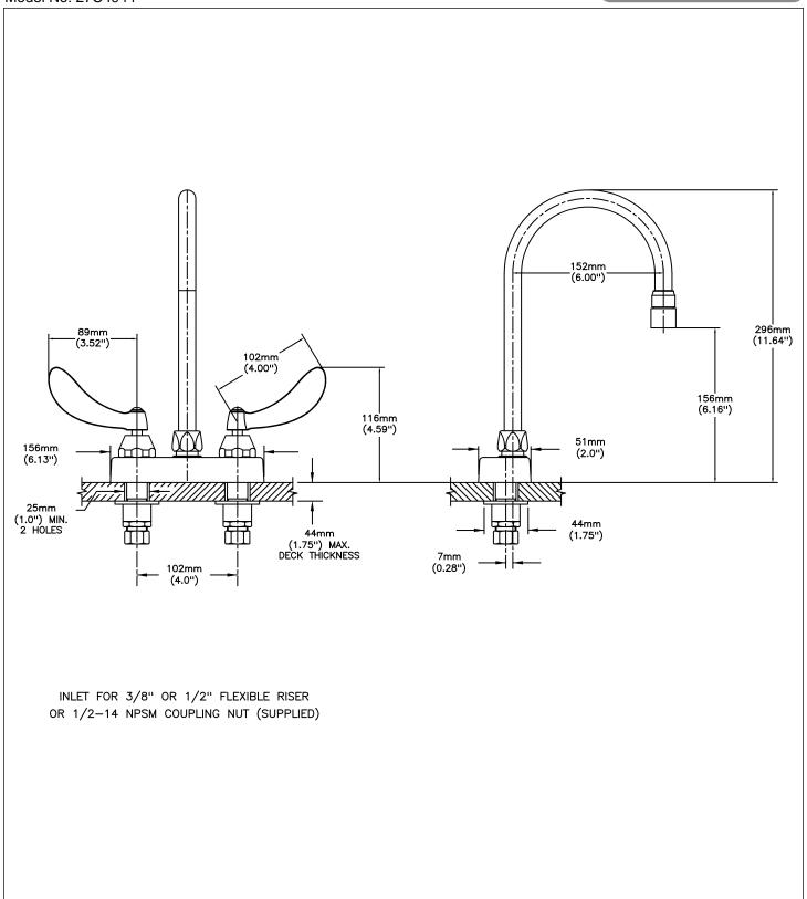
Delta reserves the right (1) to make changes to specifications and materials, and (2) to change or discontinue models, both without notice or obligation. Dimensions are for reference. Measurement may vary plus or minus 6mm(0.25"). Mounting locations are suggested only. Check with local codes for requirements in your area. This spec was produced June 09, 2014.
