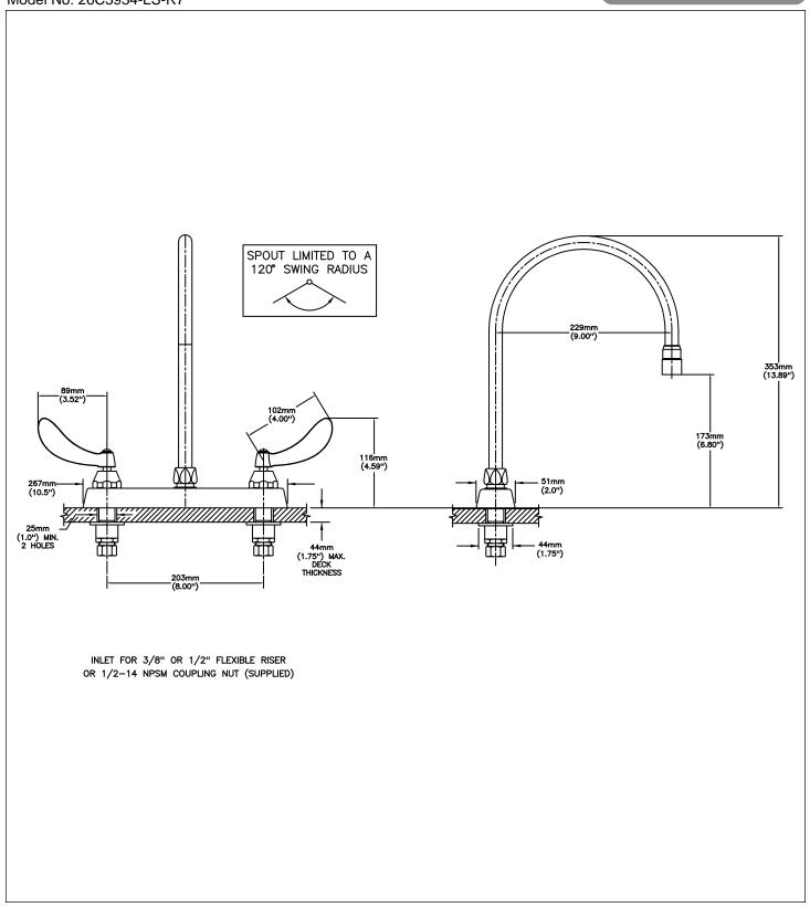
Delta reserves the right (1) to make changes to specifications and materials, and (2) to change or discontinue models, both without notice or obligation. Dimensions are for reference. Measurement may vary plus or minus 6mm(0.25"). Mounting locations are suggested only. Check with local codes for requirements in your area. This spec was produced February 15, 2013.
