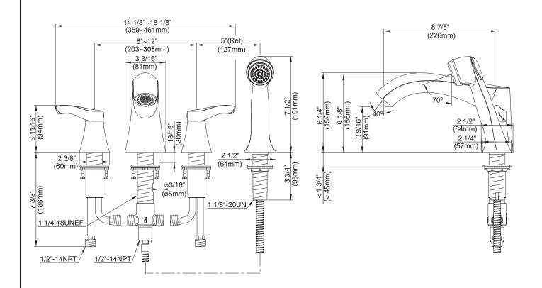
\* Danze Soft Touch Personal Shower™ is designed to operate only when the button is pressed; water will flow to the spout whenever pressure is released from the button.
