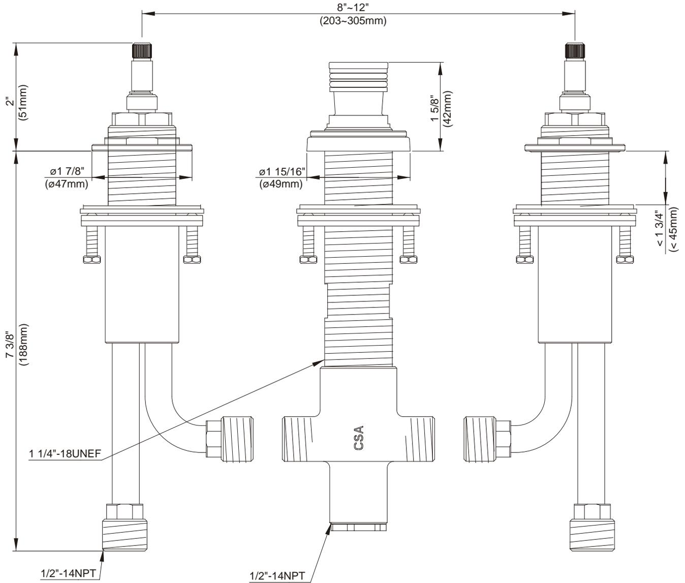
\* Installation method shown is for deck thickness of less than 1-3/4".
