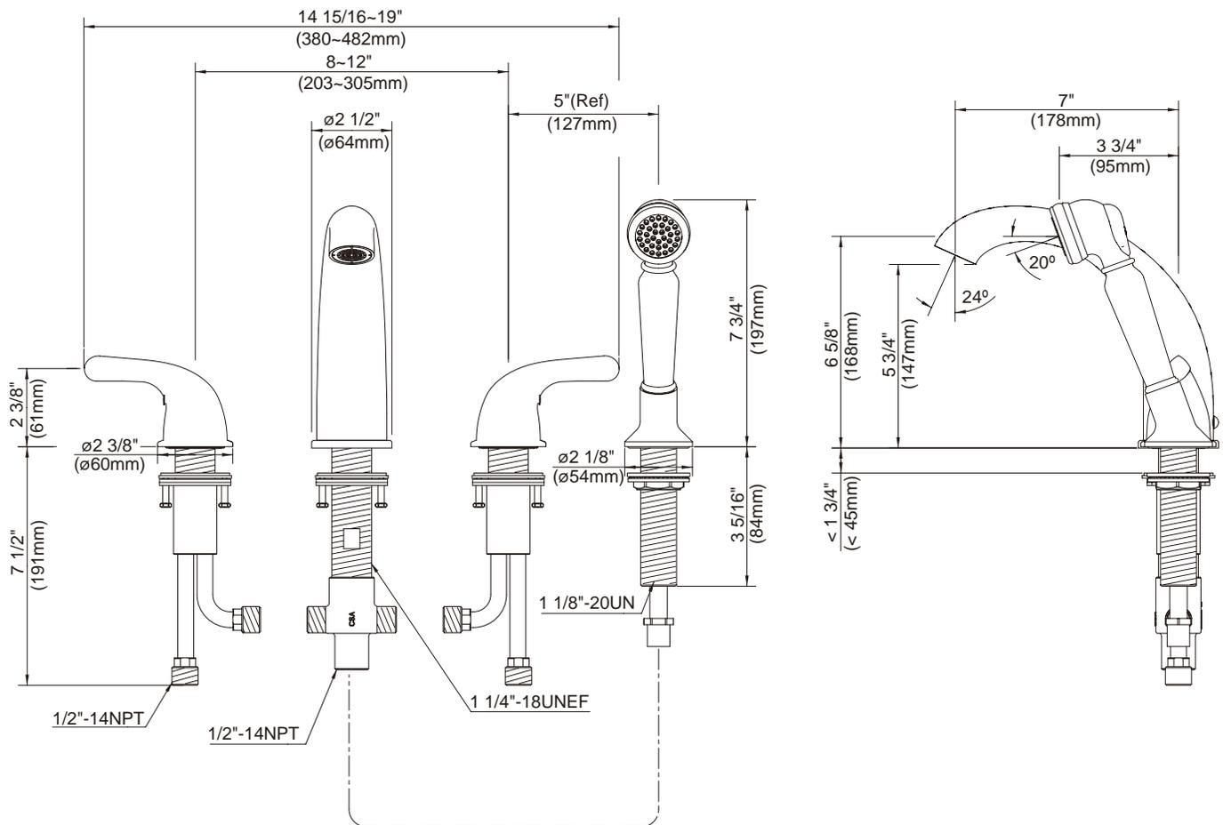
\* Danze Soft Touch Personal Shower™ is designed to operate only when the button is pressed; water will flow to the spout whenever pressure is released from the button.
