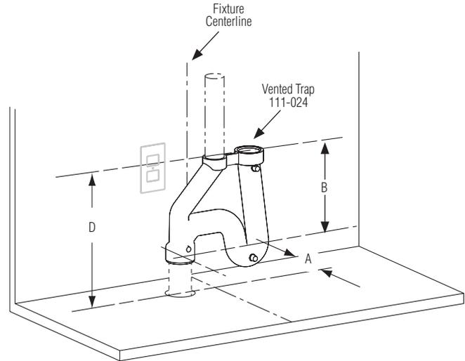
\* Suggested location of 110VAC GFCI electrical outlet. Always check local codes before installing. Outlet may be required to be in a remote location.
