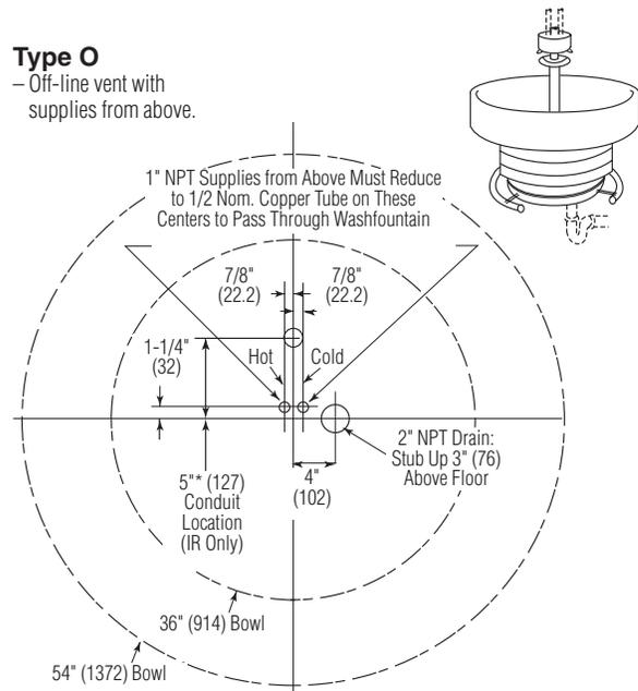
\* Remote mounting of transformer with 24 VAC electrical supply to washfountain is recommended. See local electrical codes before roughing in. (This conduit location is only a recommendation.)
