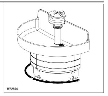
The infrared sensor uses a conical-shaped transmitting beam, having a detection area adapted to, but not exceeding, the bowl perimeter. The adaptive infrared sensor automatically adapts to the bowl after power is turned on. The infrared sensor is not affected by varying color tones or darkness. Direct sunlight or bright washroom lights will not activate the system. Infrared models also include solenoid valves and a low-voltage transformer as standard equipment:
