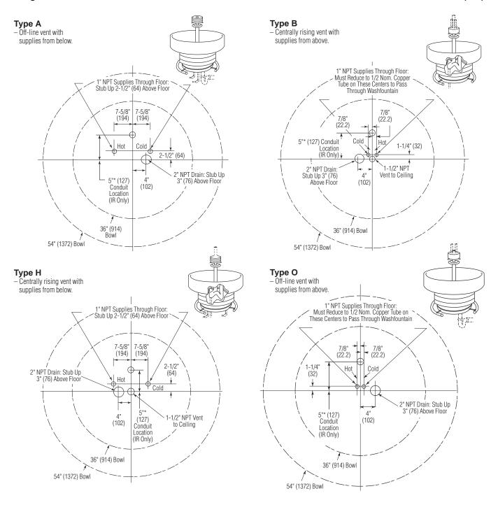
\* Remote mounting of transformer with 24 VAC electrical supply to washfountain is recommended. See local electrical codes before roughing in. (This conduit location is only a recommendation.)
