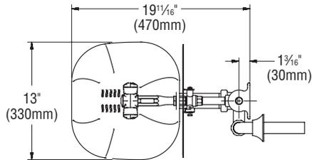
All dimensions assume standard thread engagement. Variations in manufacturing allow for +/- 1/8" (3mm) per threaded joint. To find the tolerance of a dimension, add the number of thread joints across the length of the dimension and multiply it by 1/8" (3mm).
