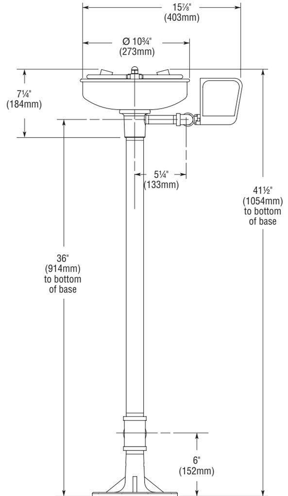
Local codes may require the installation of a backflow prevention valve to complete proper installation. Compliance with local codes is the responsibility of the installer. Valve must be tested annually to verify that it is functioning properly. Backflow prevention valves are not included with the fixture and may be supplied by the contractor or purchased from Bradley Corporation.
