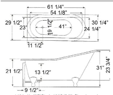
Dimensions of fixture are nominal and may vary within the range of tolerances established by ANSI Standard A112.19.1M. Dimensions and specifications subject to change without notice.
