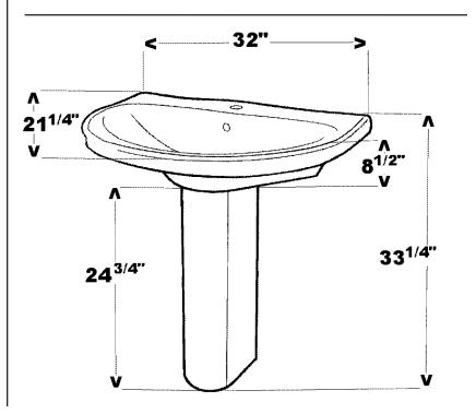
Dimensions of fixture are nominal and may vary within the range of tolerances established by ASME Standard A112.19.2-2008. Dimensions and specifications subject to change without notice.
