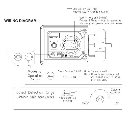
Delay Flush = User must leave the sensor range for 3 seconds before a flush is generated.
