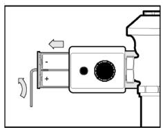
wrench to remove battery compartment side forward and out. tray.
