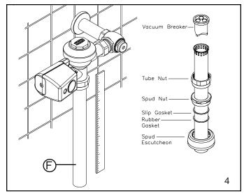
**4.)** Determine the length of vacuum breaker tube **(F)** required to join the flush valve and fixture spud. Cut the vacuum breaker tube, if required, to this length. Assemble the vacuum breaker tube assembly and spud nut assembly to the flush valve and fixture spud.
