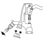
By pulling down on the diverter sleeve during flow, water will be diverted through the backflow preventer (BFP), and allow use with a hose.
