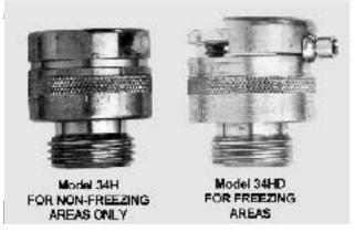
NIDEL® Model 34H anti-siphon vacuum breaker is designed to protect hose connections from contamination where temperatures do not get below freezing. Uses include laundry tubs, utility sinks, boiler room hose bibbs and outside hose bibbs in non-freezing areas.
