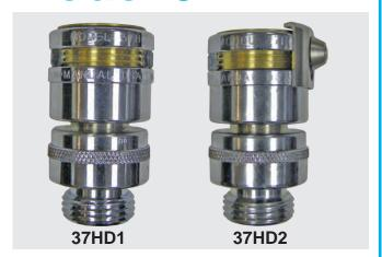
The NIDEL® Model 37HD1 / 37HD2 hose connection backflow preventers are intended for irrigation purposes and designed to protect hose connections from backflow contamination in freezing and non-freezing conditions. Manual draining is required and provides easy, sure drainage during freezing weather. Uses include outside hose bibbs, wash racks, dairy barns and swimming pool areas
