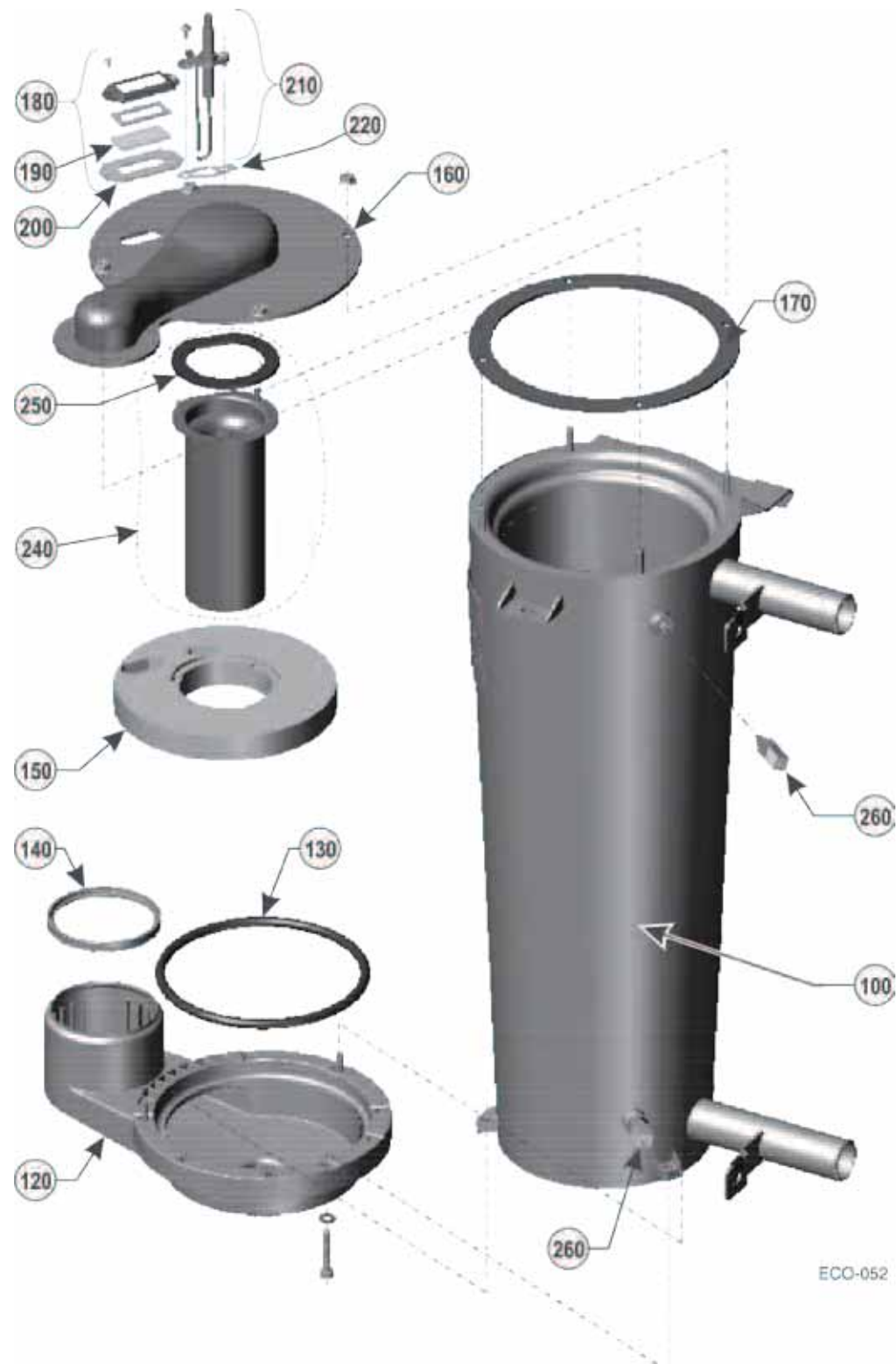
Figure 113 Heat exchanger assembly ECO 70/110 (see Figure 112, page 110 for part numbers)
