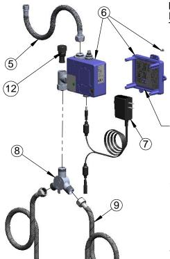
A Maximum of (8) ChekPoint Faucets can be Hardwire Connected and Powered by EC-HARDWIRE ChekPoint Hardwire AĆ Transformer. (Sold Separately)
