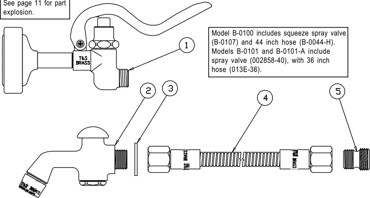
Model B-0100 includes squeeze spray valve (B-0107) and 44 inch hose (B-0044-H). Models B-0101 and B-0101-A include spray valve (002858-40), with 36 inch hose (013E-36).
