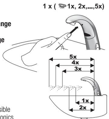
Note: Updated electronics have visible red and green LED. Original electronics have only red LED and range setting is reversed (1 = longest, 8 = shortest)
