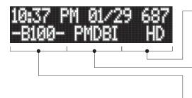
**NOTICE**: The second line will show typical reading as shown unless an error code is displayed. See codes at right.
