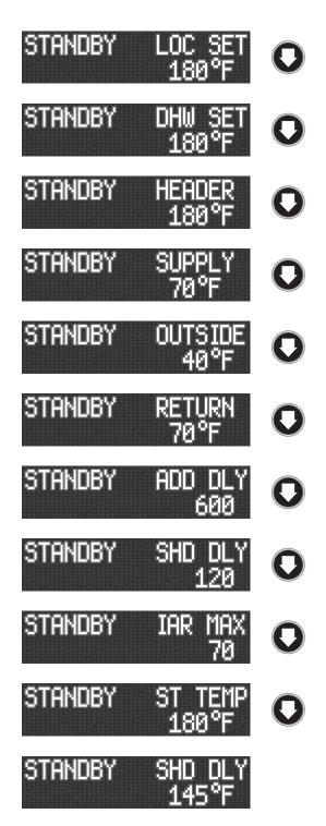
Figure 8.1: Control Display During Standby (No Call for Heat) — Pressing the DOWN Key on the Keypad Changes the Display as Shown
