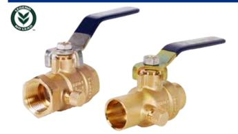
T/S-2102NL no lead brass full port ball valve with drain is ideal for maintenance and freeze protection. The EPDM O-ring and PTFE packing gland stem assures reliable and smoother operation requiring less torque. Constructed of no lead & DZR binary brass alloy. 1/2"- 1", FNPT x FNPT and 1/2"- 1", Sweat x Sweat.
