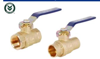
The T/S-2001NL is a smaller pattern full port ball valve designed exclusively for potable water applications in compliance with the no lead law. Constructed of no lead & DZR binary brass alloy that requires no additional steps to solder as compared to traditional brass. Available in sizes and configurations 1/2" - 2", FNPT x FNPT and 1/2" - 2", Sweat x Sweat.
