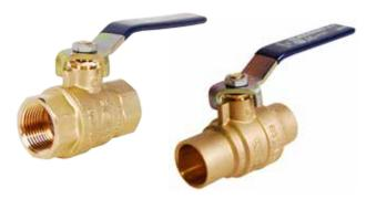
The T/S-2000 full port ball valve has a larger pattern body suitable for most any application. The EPDM O-ring and PTFE packing gland stem assures reliable and smoother operation requiring less torque to operate. The PTFE seats reduce friction thus improving the long life of the valve. The ball is chrome plated brass. The nickel plated handle is corrosion resistant. Available in sizes and configurations 1/4"- 4", FNPT x FNPT and 1/2"- 4", Sweat x Sweat.
