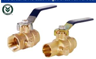
T/S-2102NL no lead brass full port ball valve with drain is ideal for maintenance and freeze protection. The EPDM 0-ring and PTFE packing gland stem assures reliable and smoother operation requiring less torque. Constructed of no lead & DZR binary brass alloy. 1/2"-1", FNPT x FNPT and 1/2"-1", Sweat x Sweat.
