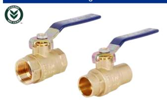
The T/S-2001NL is a smaller pattern full port ball valve designed exclusively for potable water applications in compliance with the no lead law. Constructed of no lead & DZR binary brass alloy that requires no additional steps to solder as compared to traditional brass. Available in sizes and configurations 1/2"- 2", FNPT x FNPT and 1/2"- 2", Sweat x Sweat.
