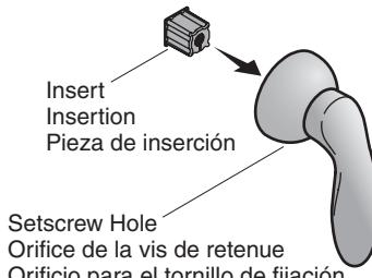
**b** Install the handle and secure with the setscrew.
