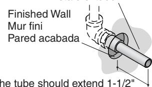
The tube should extend 1-1/2" (3.8 cm) - 2-7/8" (7.3 cm) past the finished wall.
