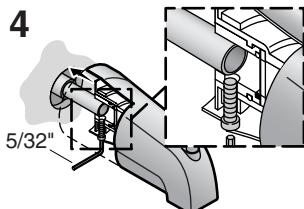
Loosen the setscrew and slide the spout against the wall.
