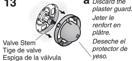
**b** Turn the valve clockwise to the full open position.
