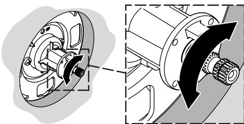
**18** Reinstall the collar with the setscrew against the tab.
