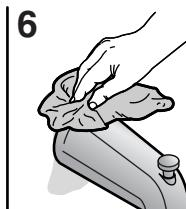
Remove the excess sealant.
