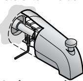
Overtightening may damage copper pipes!
