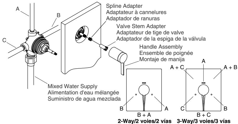
**NOTE: Valve Operation.** Water will flow from a single shower accessory when the control knob detent lines up with any of the markings on the escutcheon. Water will flow from two accessories at the same time when the control knob detent is midway between the markings.
