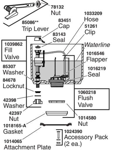
78132 Nut<br>85086** Trip Lever<br>83451 Cap<br>83143 Seal<br>1033209 Hose<br>51261 Clip<br>1039862 Fill Valve<br>85307 Washer<br>84678 Locknut<br>42398 Washer<br>42397 Nut<br>1018165-A Gasket<br>1014065 Attachment Plate<br>1060218 Flush Valve<br>1016546 Flapper<br>1016219 Seal<br>1014580 Nut<br>1024390 Accessory Pack (2 ea.) |
