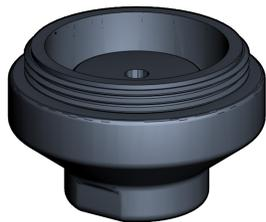
3. **Inspect Flow Control(s).** Each spray head contains a flow control to regulate the flow of water through the spray head. The flow control assures that the unit delivers a soft, generous flood of water regardless of incoming water line pressure. Over time, debris can collect in the flow control or it can deteriorate due to age. If this occurs, the flow control must be cleaned or replaced. ***Inspect flow control for debris and/or deterioration. Clean or replace as required.***
