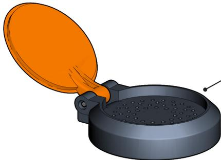
1. **Inspect “Flip Top” Dust Cover(s).** Guardian developed the “flip top” style dust cover as an alternative to the loose caps with chains that other manufacturers use. The “flip top” cover is attached to the spray head by a permanent stainless steel rivet so it can never be lost or removed. ***Verify that the cover swings freely and is removed from the spray head by the water flow.***
