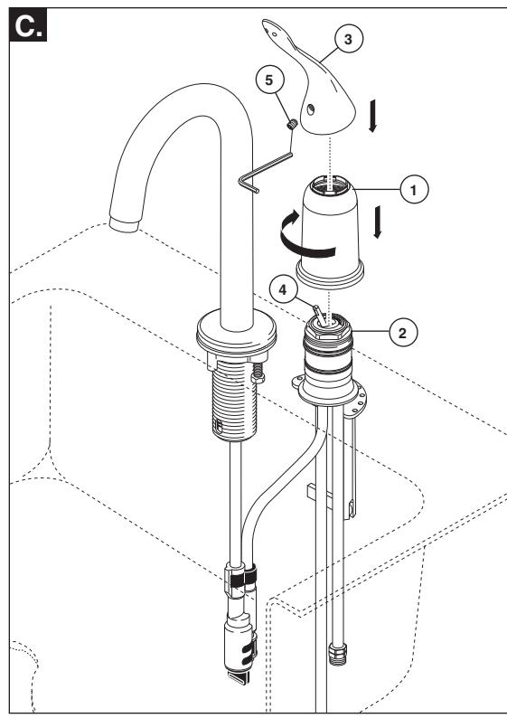
**C.** Thread sleeve (1) over bonnet (2) and hand tighten. Place handle (3) on stem (4) and secure with set screw (5).
