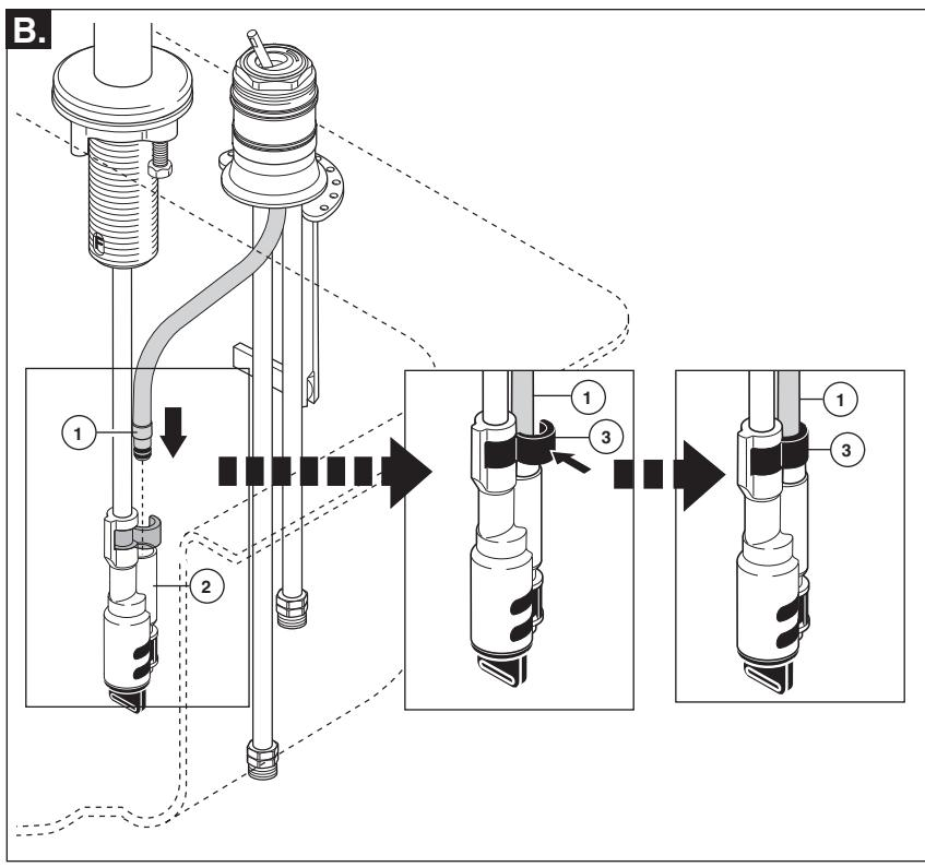
**B.** Slide tube end (1) into adapter (2) and secure with clip (3). Pull moderately on tube to ensure connection has been made.
