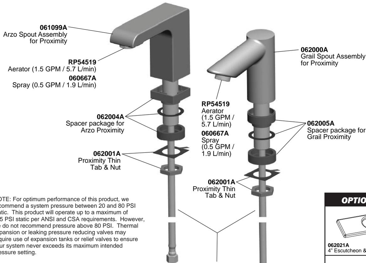
NOTE: For optimum performance of this product, we recommend a system pressure between 20 and 80 PSI static. This product will operate up to a maximum of 125 PSI static per ANSI and CSA requirements. However, we do not recommend pressure above 80 PSI. Thermal expansion or leaking pressure reducing valves may require use of expansion tanks or relief valves to ensure your system never exceeds its maximum intended pressure setting.
